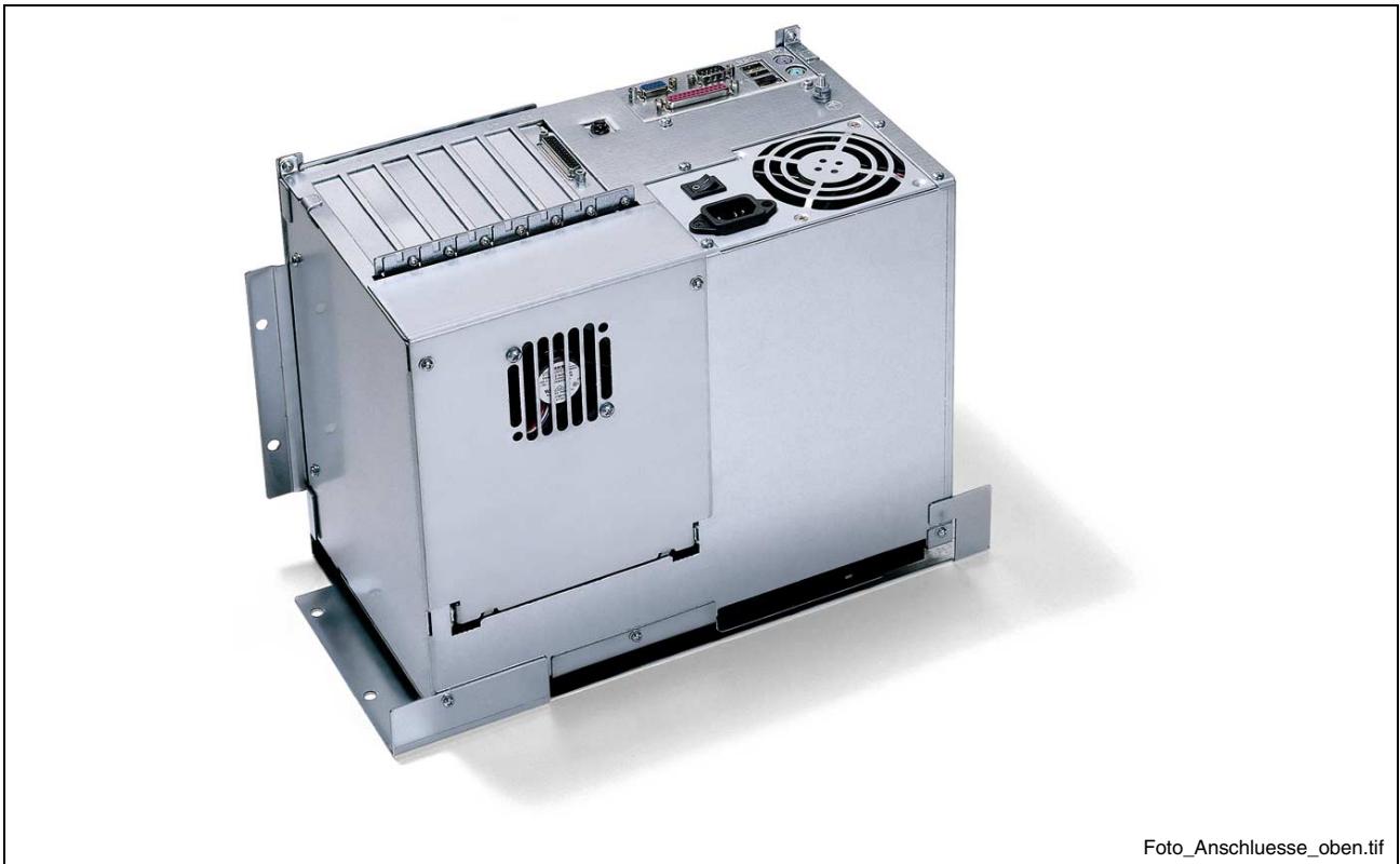
Fig. 5-5: Connector panel on the top side, optional drive in forward direction
