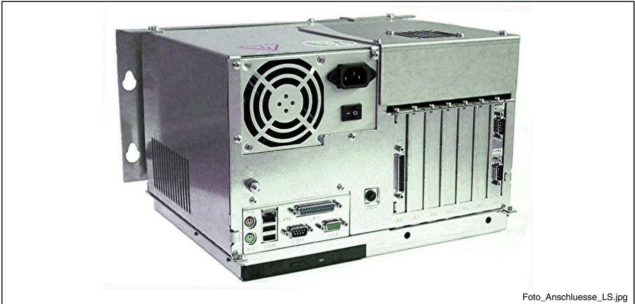
Fig. 5-7: Mounting with connector panel in forward direction
