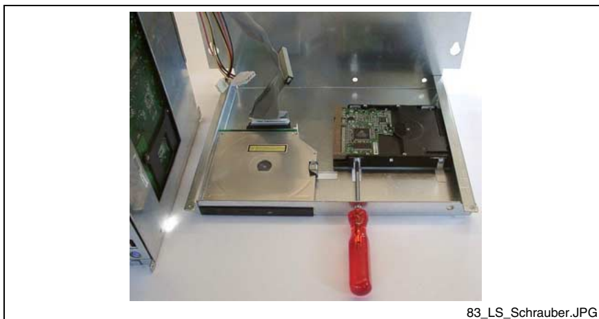
Fig. 8-10: Loosen the fastening screws of the hard disk
