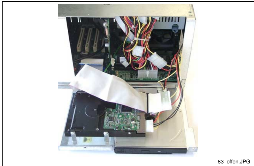
Fig. 8-5: Lifted hard disk frame
