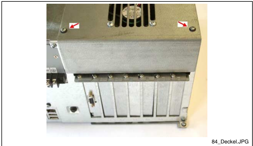
Fig. 8-11: Loosen the fastening screws of the cover
