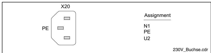
Fig. 7-15: Pin assignment of the 230/115 VAC connection X20
