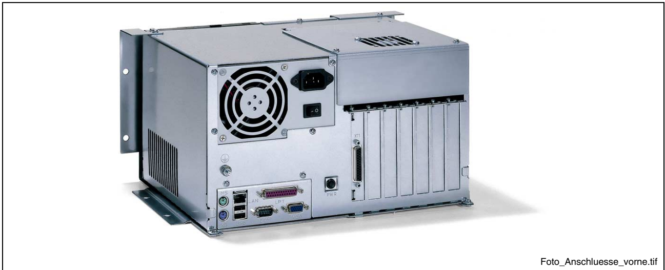
Fig. 5-3: Connector panel in forward direction, optional drive at the top
