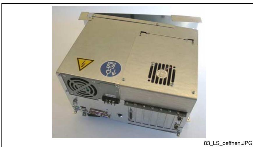
Fig. 8-7: Loosen the VSB 40.1 from the mounting plate
