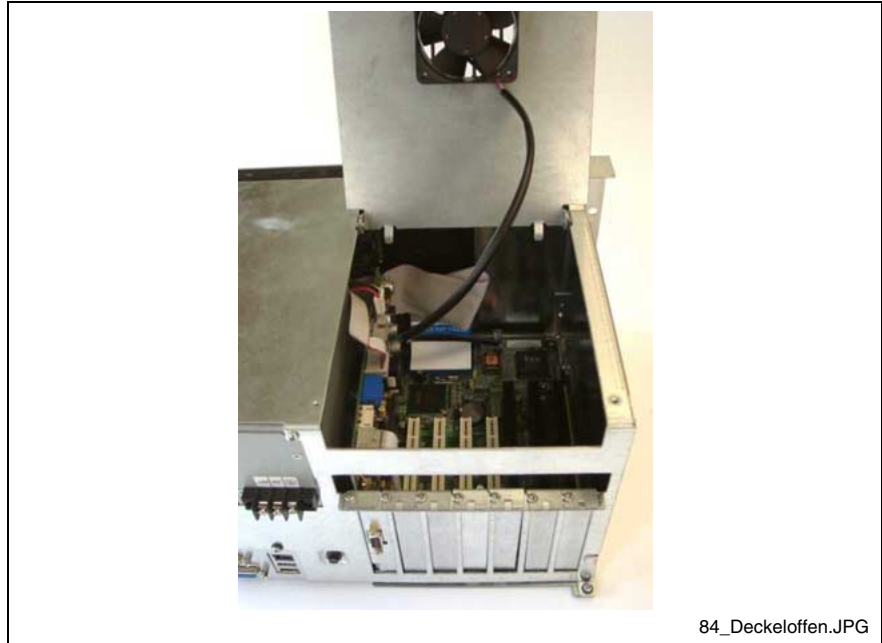
Fig. 8-12: Lift the cover with fan
