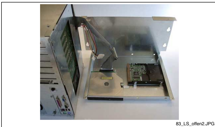
Fig. 8-9: Loosen the cable from the hard disk
