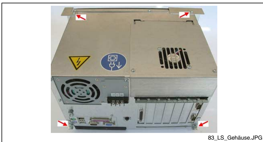
Fig. 8-6: Loosen the fastening screws at the mounting frame
